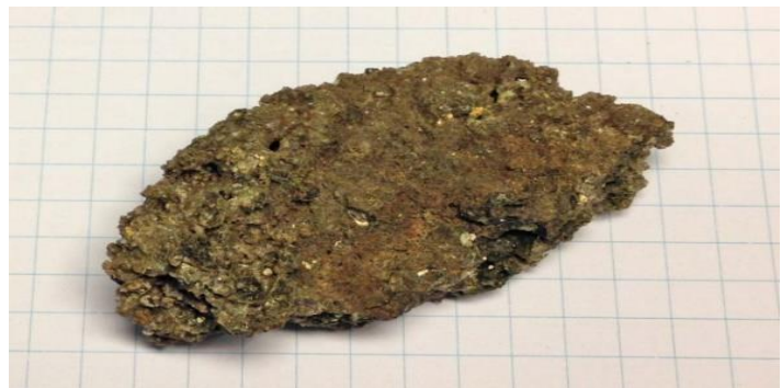
Figure 6: Sintered ashes from the first 100% used bedding gasification test (squares on the paper are 5 mm).
